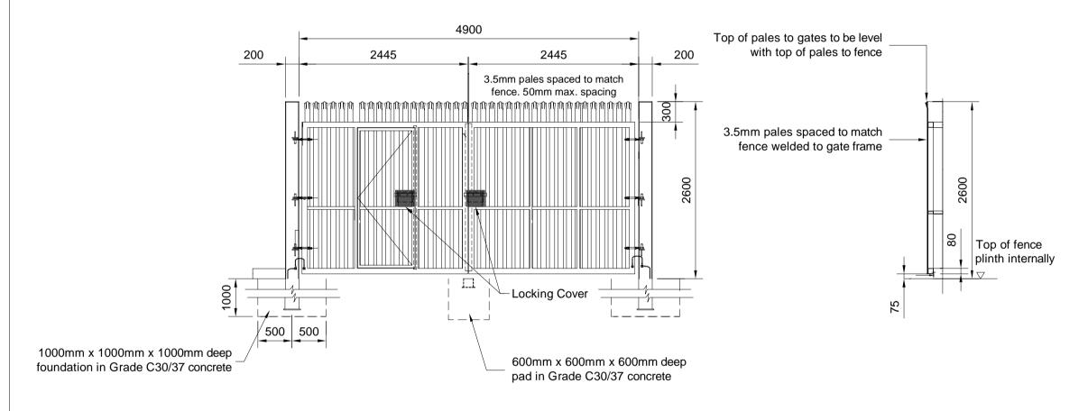
SECURITY FENCE(PALISADE) GATE ELEVATION
